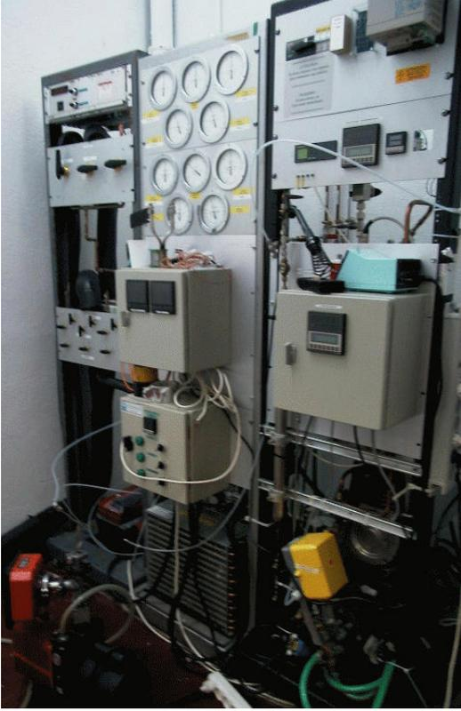
Fig. 1. Photography of the evaporative cooling plant used at CPPM; see fig. 5 for a schematical view. Compressor and condenser can be recognized at the lower right border. Connections to the pixel stave are positioned at the left side of the rack.
