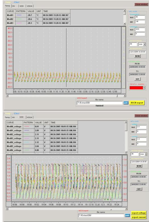
Fig. 8. Automatic temperature cycling run, seen in the temperature monitoring (top) and voltage and current monitoring panel (bottom)
